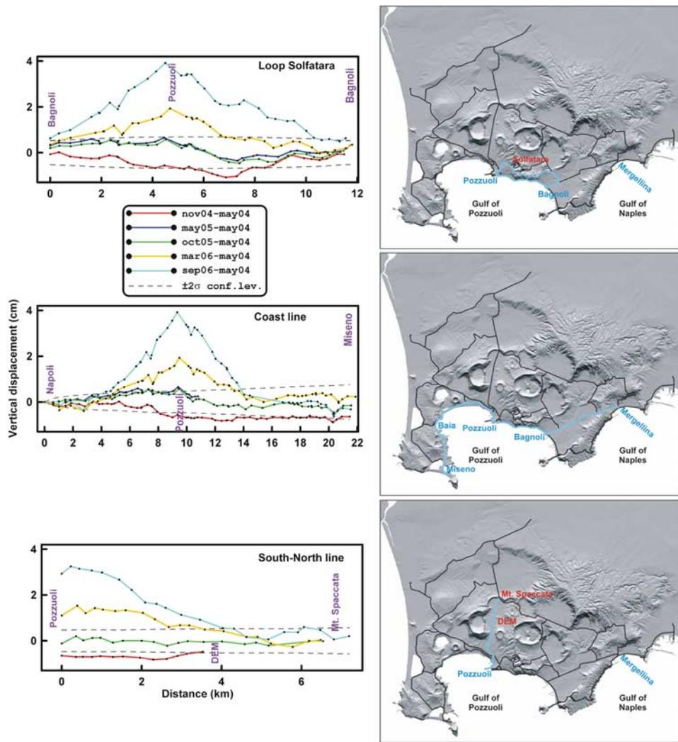
**Figure 2.** Recent vertical displacements from precision levelling. Vertical displacements measured along three levelling lines during different periods, since May 2004 to September 2006, as indicated in figure. Displacements are all referred to the benchmark of Mergellina.  $2\sigma$  confidence levels are indicated. Ground uplift starts in November 2004, reaching up to 4 cm in September, when last levelling measures were made.
